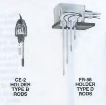
TYPE B electrode rods are 1/4" diameter and are tapped 6-32 for use only on Type CE-2 and CE-3 holders. Lengths over 12 inch should be insulated and lengths over 30 inch not recommended.
