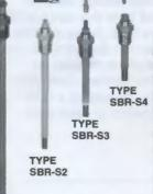
BIW offers a variety of these small electrode assemblies to meet special OEM situations for single electrodes. The bushing has a 1/4" NPT SBR-S4 inc. and in pressure-tight mounting and is available in either cadmium plated steel or 316 S.S. The electrode rod is 1/4" O.D. and must be insulated for at least 1" below the bushing. The available PVC or teflon insulated rod materials are listed on page 2. There is a choice of four methods to connect the electrode lead wire
